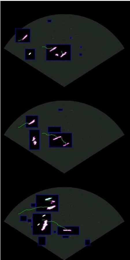
Fig. 7. Kalman filter tracking (real data).
