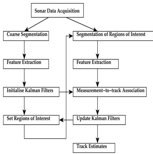
Fig. 1. Kalman Filter Tracking Procedure.
