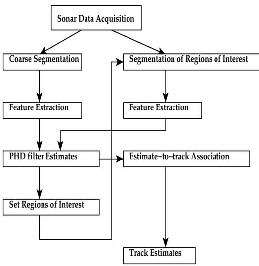
Fig. 2. PHD Filter Tracking Procedure.
