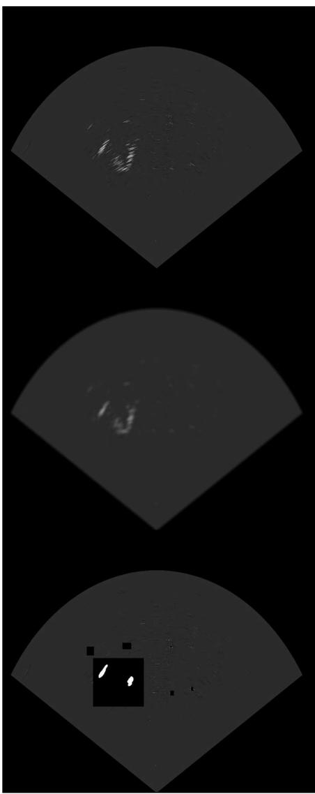
Fig. 4. Original sonar image (left). Image after filtering (middle). Resulting image after segmentation with regions of interests shown as the boxes and potential targets as the white segmented areas (right).
